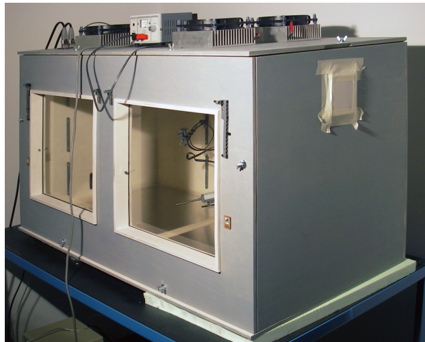
Figure 3.1: Thermal Model house: a portable experimental test facility for building physics studies, developed by UdK Berlin.
